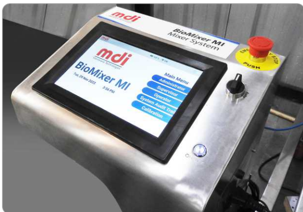
Control panel with capacitive touch screen display
