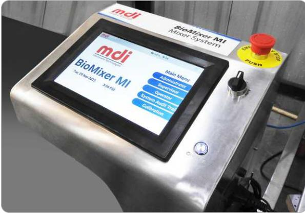
Control panel with capacitive touch screen display
