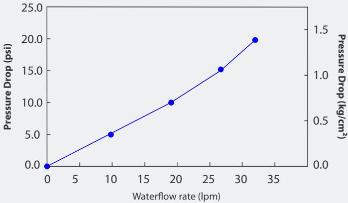
**0.2µm AseptiSure® WS, 10" Standard Cartridge Filters**
