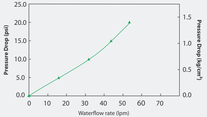
**0.2µm AseptiSure® WS, 20" Standard Cartridge Filters**
