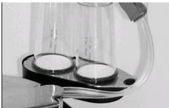
**Pic. 3: Stericheck canisters placed on the drain tray**
