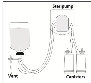
**Pic. 5: Schematic Set-up of Stericheck LVP**
