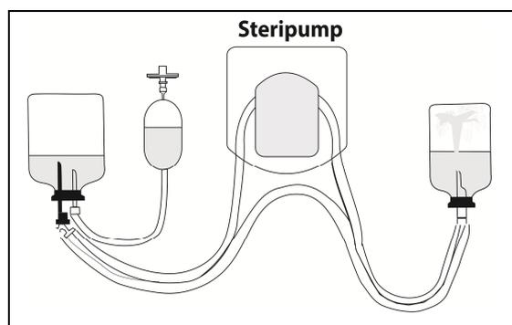
**Pic. 4: Schematic Set-up of Stericheck SVP Dilutor**
