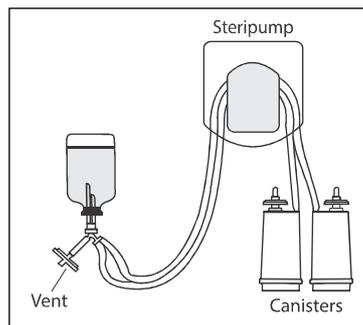
**Pic. 5: Schematic Set-up of Stericheck SVP1**
