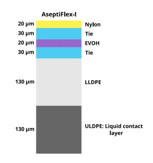
Biocompatibility for media storage and cell growth: AseptiFlex film is made of plastics of Non Animal Origin and is validated for Biological Reactivity tests as per USP
